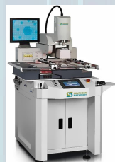
BGA Rework Station
